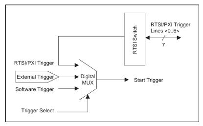
Figure 2-4. Waveform Generation Trigger Sources
